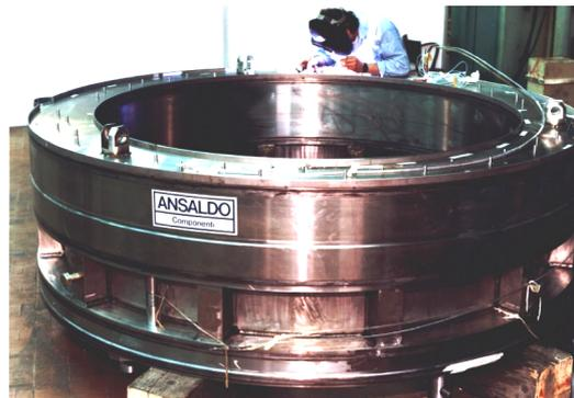
*S.C. coils during assembly of the cold mass*
