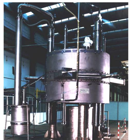
*AGOR cryostat during factory cold test*
