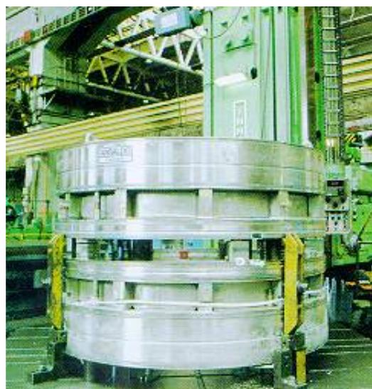
*Machining of the cold mass after seal welding*
